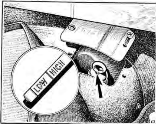
Fig. P.11. The gearbox dipstick.
