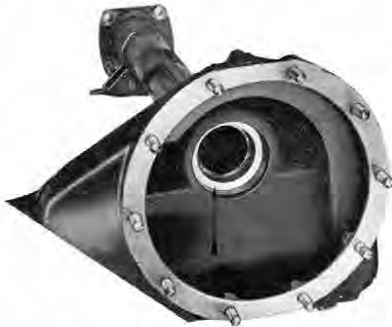
Fig. H.12. The location of the pinion bearing spacer in the axle casing is indicated by the arrow.
