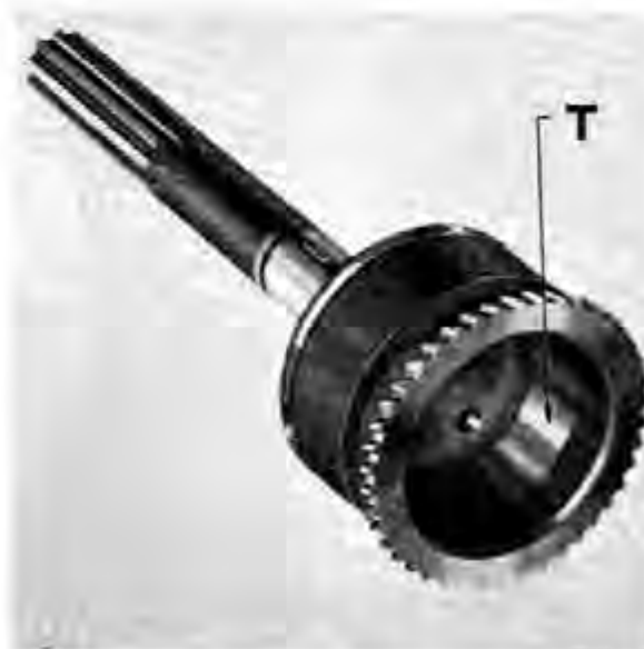
Fig. FFF.9. The output shaft. Note the outer race "T" of the free-wheel.
