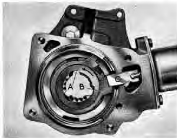
Fig. FFF.11. Pawl before engagement. As the control plate rotates, see arrow, the blocker ring latches the pawl against forward movement.
