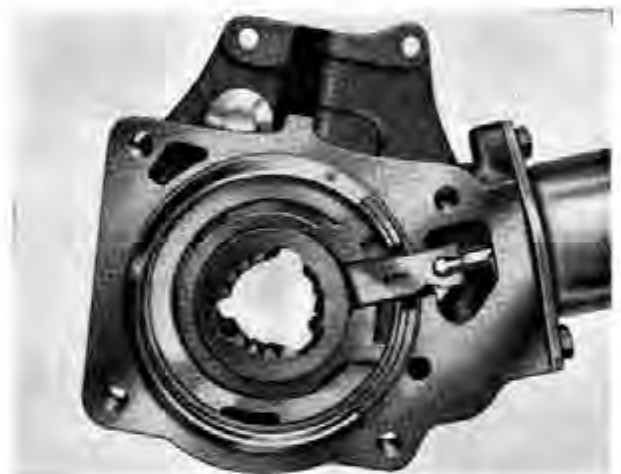
Fig. FFF.12. Pawl engaged. The control plate has reversed its rotation just sufficiently to unlatch the spring-loaded pawl, which has snapped forward and locked the control plate.
