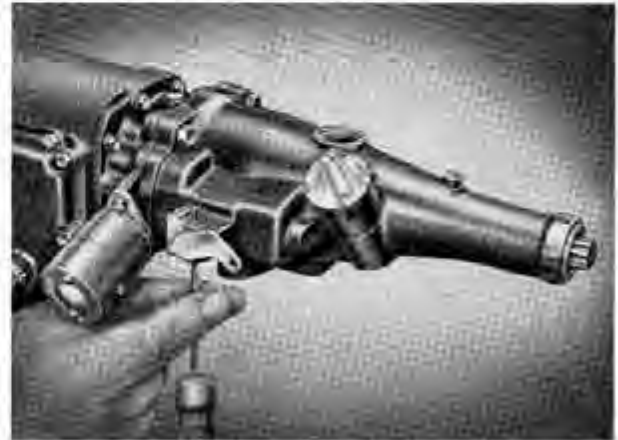
Fig. FFF.19. Removing the taper pin which holds the control lever in place.
