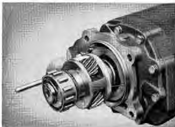
Fig. FFF.18. Overdrive body removed, leaving adaptor plate and gears on the gearbox. The clutch rollers are held in position for assembly with a minimum of thick grease.
