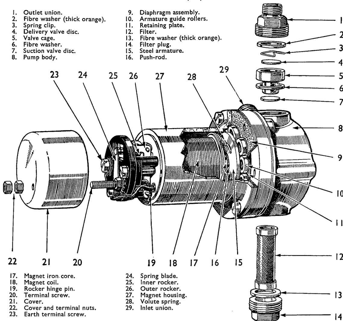
Clean the filter in fuel with a brush and swill out the body of the pump.
